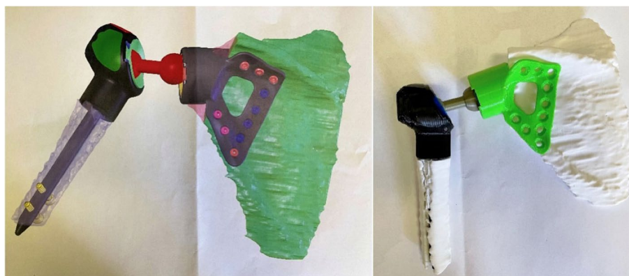
Fig. 3 Preliminary 3D-printed dummy. Pictures demonstrating the initial design and printed dummy subject to team approval prior to definitive surgery. Dumbbell connector linking the humeral and scapular components
